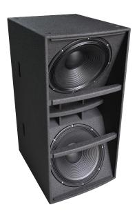
VH Sub218R is a special Sub-Bass unit housing two long excursion 18in. direct radiating transducers mounted in two separated Bass-refex tuned enclosures. It consists of two coupled VH Sub118R with one physically facing up in the cabinet bottom side.
